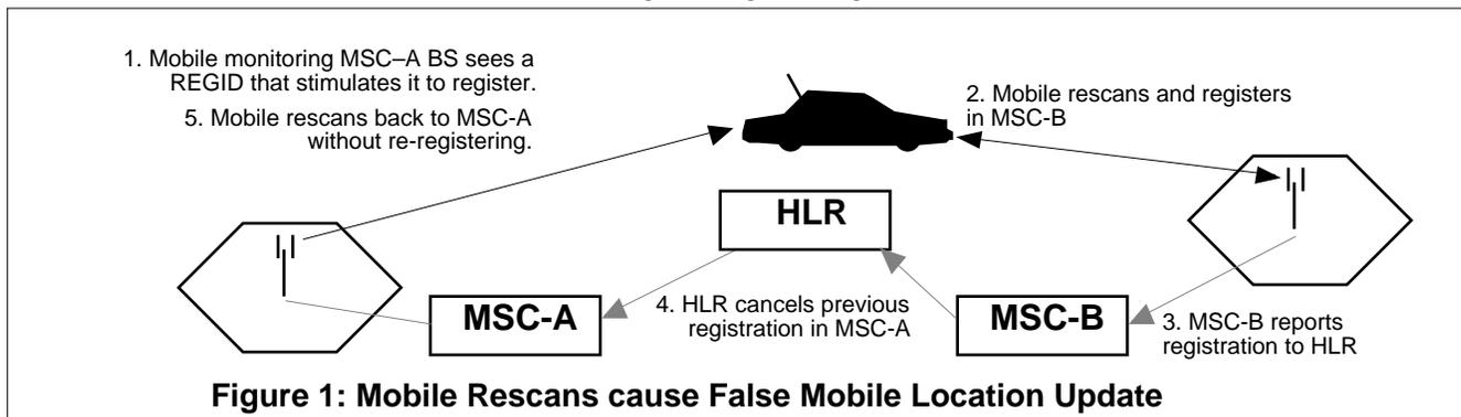
Figure 1: Mobile Rescans cause False Mobile Location Update
